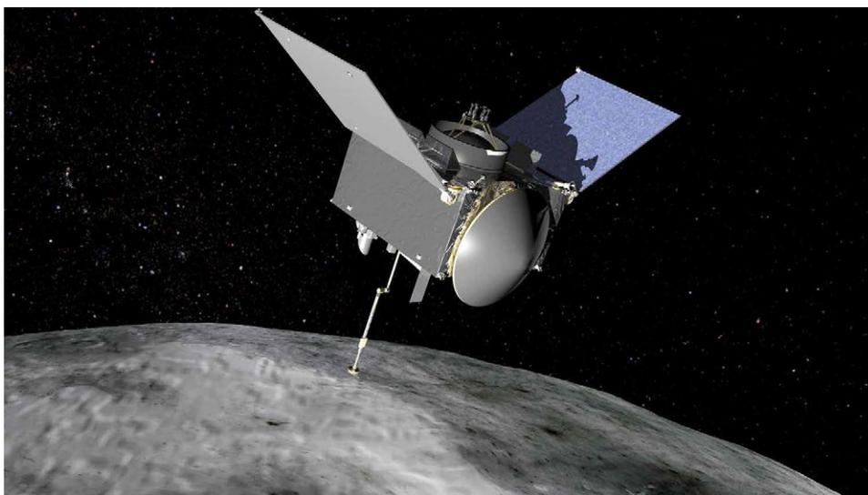
Fig. 2. OSIRIS-REx spacecraft with the TAGSAM robotic sampling arm (courtesy of NASA).
