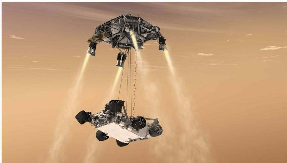
Fig. 4. Mars 2020 rover being deployed by Skycrane (courtesy of JPL/NASA).
